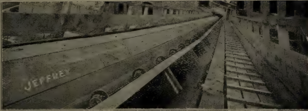
Jeffrey Cable Conveyor handling Pulp Wood between buildings in Paper Mill
